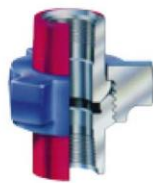
Hammer UNION type 1502 with NPT thread connection - Pressure Rating: 15,000 psi
