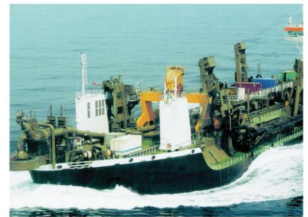
Trailing suction hopper dredgers
