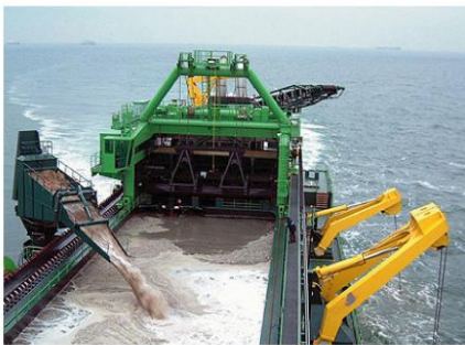
Stationary suction dredger
