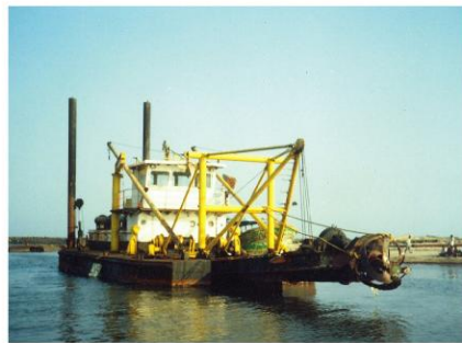
Cutter suction dredger
